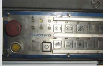
This device is a switch or button on the blank side of each section that when activated on the second cycle puts the IS machine section into swab mode.
