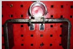
This device is placed on the invert rack to prevent the neck-ring arm from reverting.
