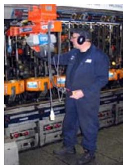
Figure 4: Fixed Lifting Equipment
