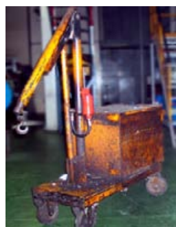
Figure 3: Mobile Lifting Equipment
